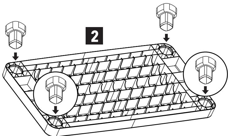
**2.** Adjust the 4 included support bases inside the couplings already installed as indicated in figure 2.
