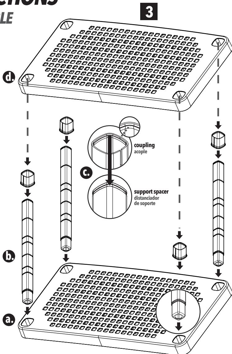
**3. a.** Put the shelf by its top side. **b.** Take 4 of the support spacers and fix them pressing down inside the 4 couplings placed in the 4 holes of the shelf as shown in figure b. **c.** Then install next 4 couplings set in the top slot of each support spacer. You will listen a clic once it is fixed. See figure c. **d.** Put on the support spacers already installed next shelf and repeat steps explained until you finish assembly of shelving.
