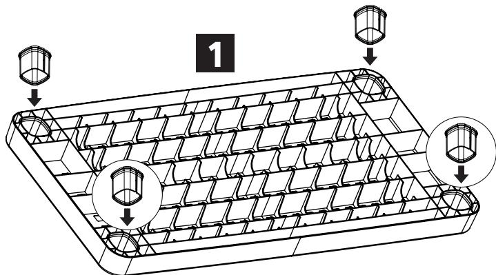
**1.** Take one of the shelves from its back part to start the assembly of the shelving. Begin from bottom to top placing the included couplings in the holes located at the end of the shelf as shown in figure 1.
