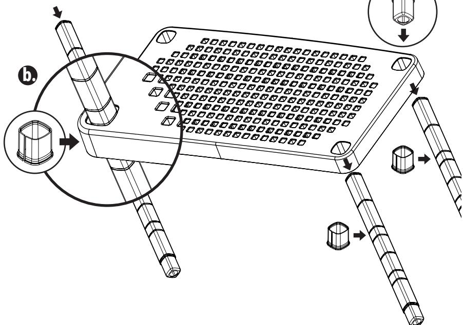
1. To use the shelving to suit your needs, just locate couplings at same distance between any of 6 slots as shown in figure a. Follow the assembly instructions detailed in point 3. This option allows you to locate the shelves in different heights getting modular spaces.
