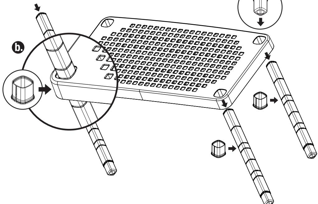
1. To use the shelving to suit your needs, just locate couplings at same distance between any of 6 slots as shown in figure a. Follow the assembly instructions detailed in point 3. This option allows you to locate the shelves in different heights getting modular spaces.
