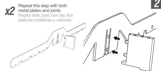
Be sure to align the metal plates with covers and holes on the sides of the pieces for later screws installation.
